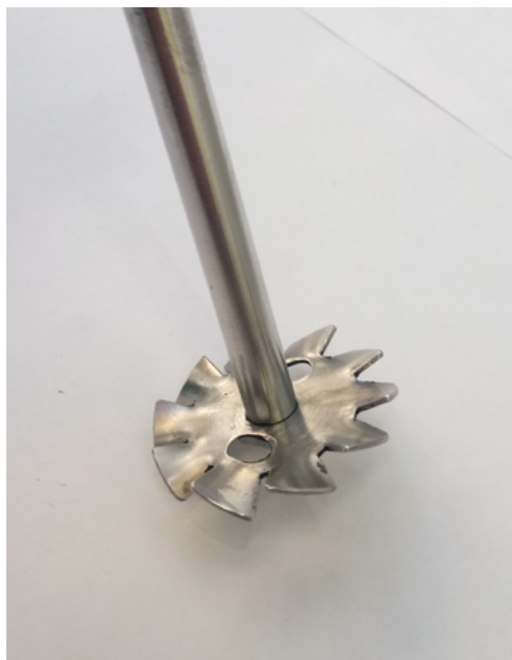
Figure 5. Recommended impeller blade shape
