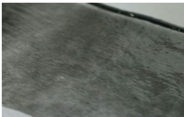
Figure 10. “Good” quality dispersion (homogeneous mixture)
