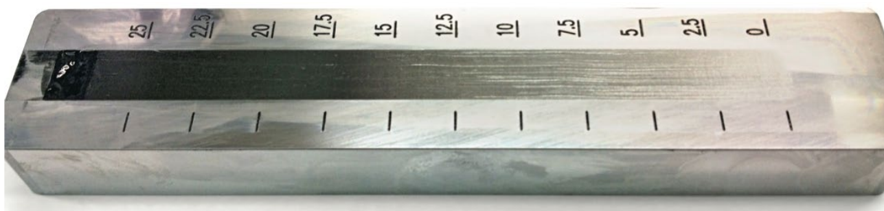
Figure 11. “Good” quality dispersion (particle size \leq 15 \mu\text{m} )
