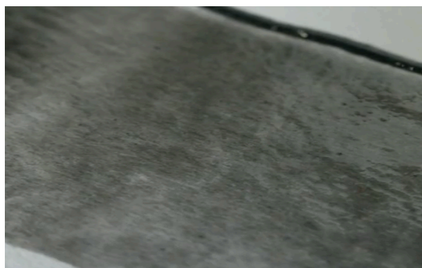
Figure 7. “Good” quality dispersion (homogeneous mixture)
