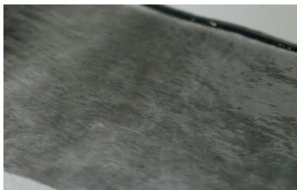
Figure 8. “Good” quality dispersion (homogeneous mixture)
