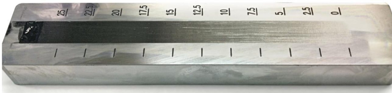
Figure 9. “Good” quality dispersion (particle size \leq 15 \mu\text{m} )
