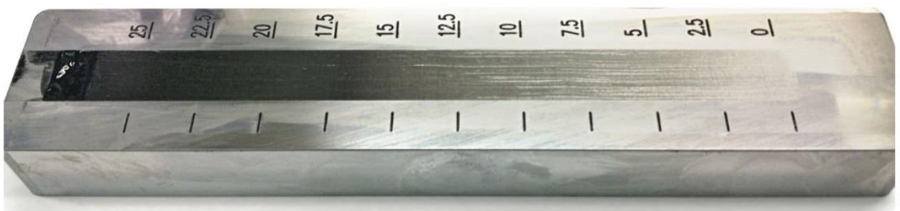
Figure 8. “Good” quality dispersion (particle size \leq 15 \mu\text{m} )
