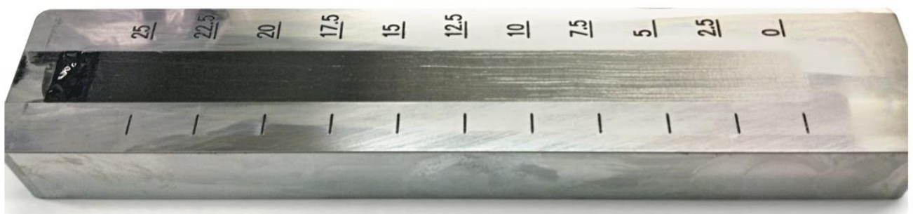
Figure 11. “Good” quality dispersion (particle size \leq 15 \mu\text{m} )
