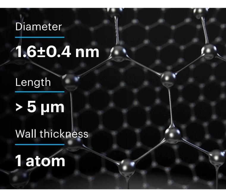
These are referred to as single wall carbon nanotubes or graphene nanotubes. Each one is a tube with a wall the thickness of a single atom of carbon, a diameter of about 1.6 nm, and a length of about 5 microns. And it can be used as a conductive agent to provide electrical conductivity to different polymer matrixes.
