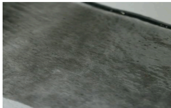
Figure 7. “Good” quality dispersion (homogeneous mixture)
