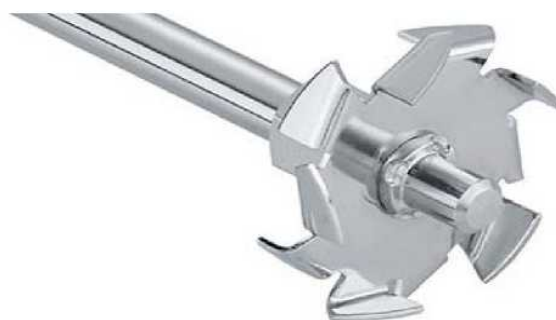
Figure 2. Recommended impeller blade shape.
