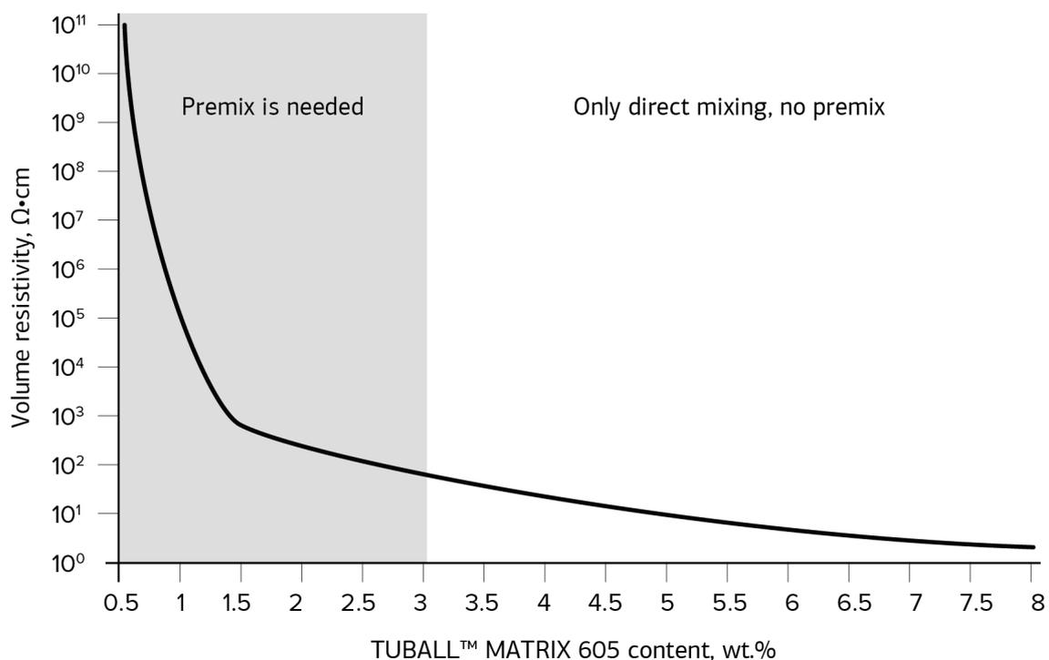
**Figure 1.** Volume resistivity of 60 Hardness HCR silicone (ELASTOSIL® R 401/60) with TUBALL™ MATRIX 605 in the range 10–10<sup>11</sup> Ω·cm (sample shape: compression-moulded rubber sheet of 2 mm thickness, compounded on two-roll mill)
