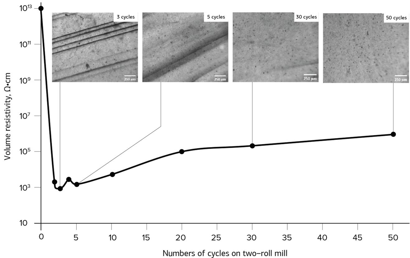
**Figure 3.** Correlation of volume resistivity, number of cycles on a two-roll mill and TUBALL™ MATRIX 605 distribution, TUBALL™ MATRIX 605 content — 0.8 wt. %
