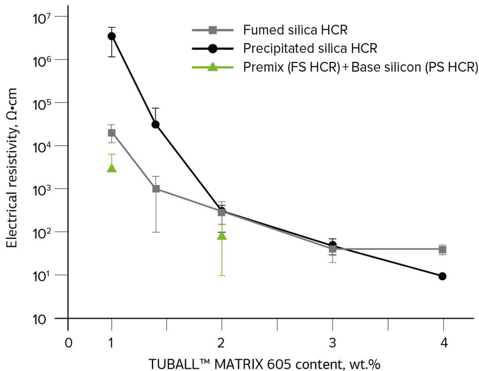
**Figure 2.** Volume resistivity of two types of 60 Hardness HCR silicone (Fumed silica based and Precipitated silica based) with TUBALL™ MATRIX 605 in the range 10<sup>1</sup>–10<sup>7</sup> Ω·cm (sample shape: compression-moulded rubber sheet of 2 mm thickness, compounded on two-roll mill)
