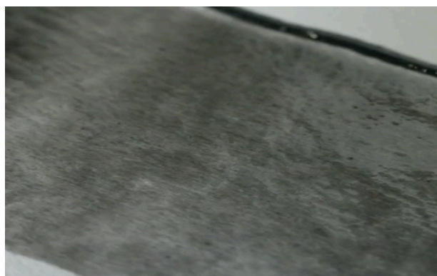
Figure 8. “Good” quality dispersion (homogeneous mixture)
